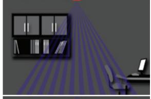
Passive infrared operates by detecting changes in temperature within a cone-shaped area around the detector.
