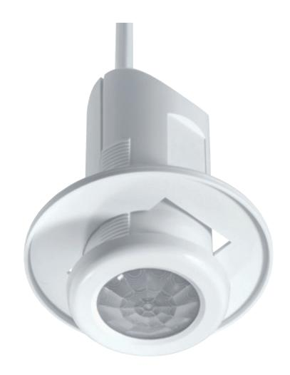
Cone shaped detection pattern. Optimum mounting height of 2.4m, gives a detection diameter of 6m Quick fixing clamp (flush mounted) adjusts to the ceiling tile thickness
