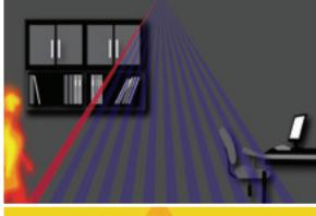
Changes in temperature within the detection area are recognised as occupancy signals.
