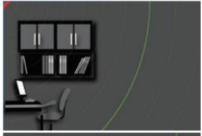
Ultrasonic and microwave detectors operate by constantly sending out signals to detect activity in the area.
