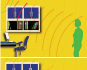
When movement is detected, this causes a distortion of the signals and the detector switches the lights on.
