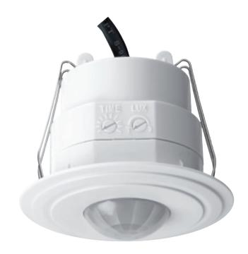
Cone shaped detection pattern. Optimum mounting height of 2.4m, gives a detection diameter of 6m
