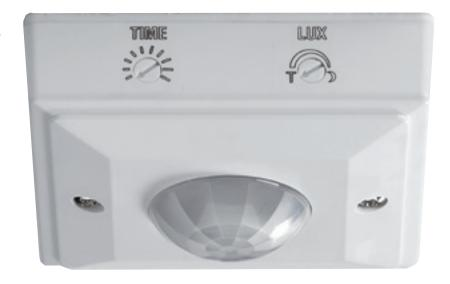
Cone shaped detection pattern. Optimum mounting height of 2.4m, gives a detection diameter of 6m
